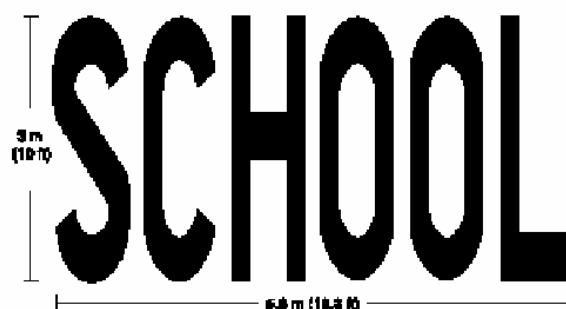
Figure 7C-1. Two-Lane Pavement Marking of "SCHOOL"
